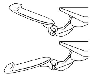
To adjust the height of the tray up and down, push down on the back of the tray while lifting the front.
