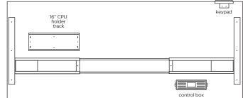
Please note: on a 48" wide desktop, the CPU Holder is best mounted behind the crossbar with the track parallel to the back edge of the desktop.
